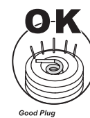
Good Plug Element glows when tested.
